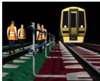
Barrier set at 4 ft (1.25m) from running rail for lines speeds up to and including 100 mph
