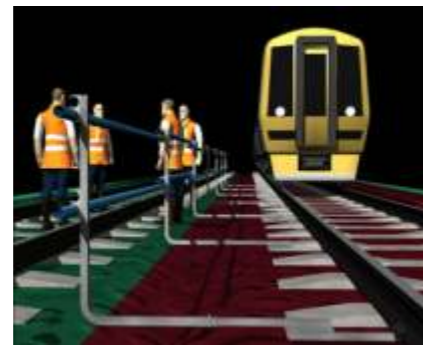
Barrier set at 6 ft6" (2m) from running rail for lines speeds over 100 mph
